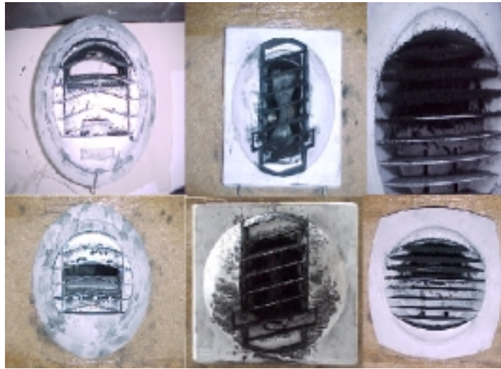
photo 1. Example of artificially loaded exhaust terminal (self-regulating).
