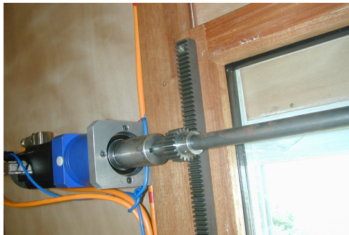
Figure 11 : View of the shaft, toothed rack and pinions
