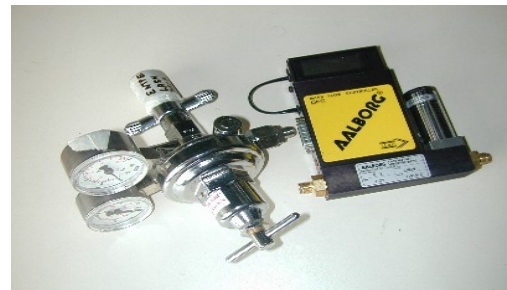
Figure 14 : Views of CO 2 injector
