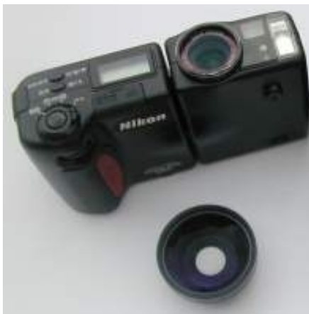
Figure 1: The Nikon Coolpix 990 and the fish eye lens FC-E8 used in this study.
