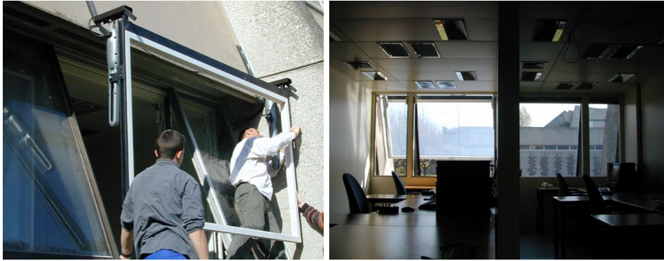
Figure 12 - Real 1:1 scale experiment within the TwinCells (right). Left Room is equipped with tiltable Serraglaze window (left).
