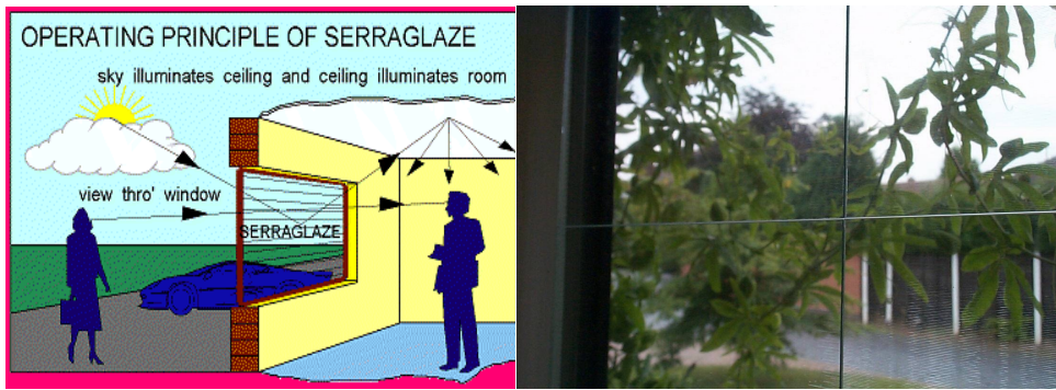
Figure 3 - Operating principle of the Serraglaze product (left), and view through the window (right).
