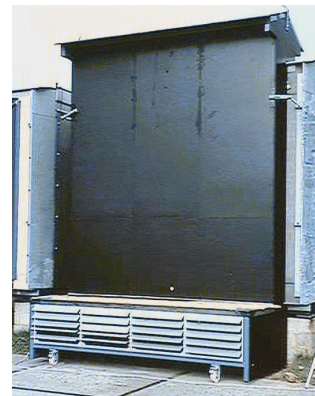
Figure 1: (a) PASLINK test cell with translucent component, (b) Outdoor cold box
