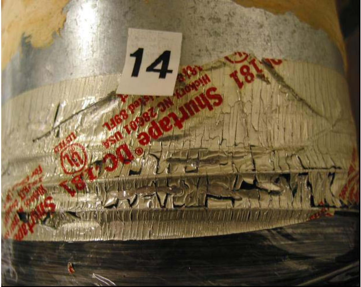
Figure A17. Sample 14. This sample shows the same cracking and splitting as Sample 13.
