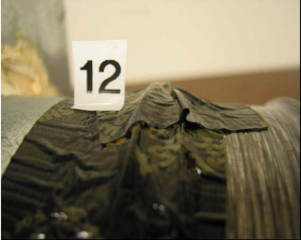
Figure A14. Sample 12. The end of the tape has wrinkled and shrunk.
