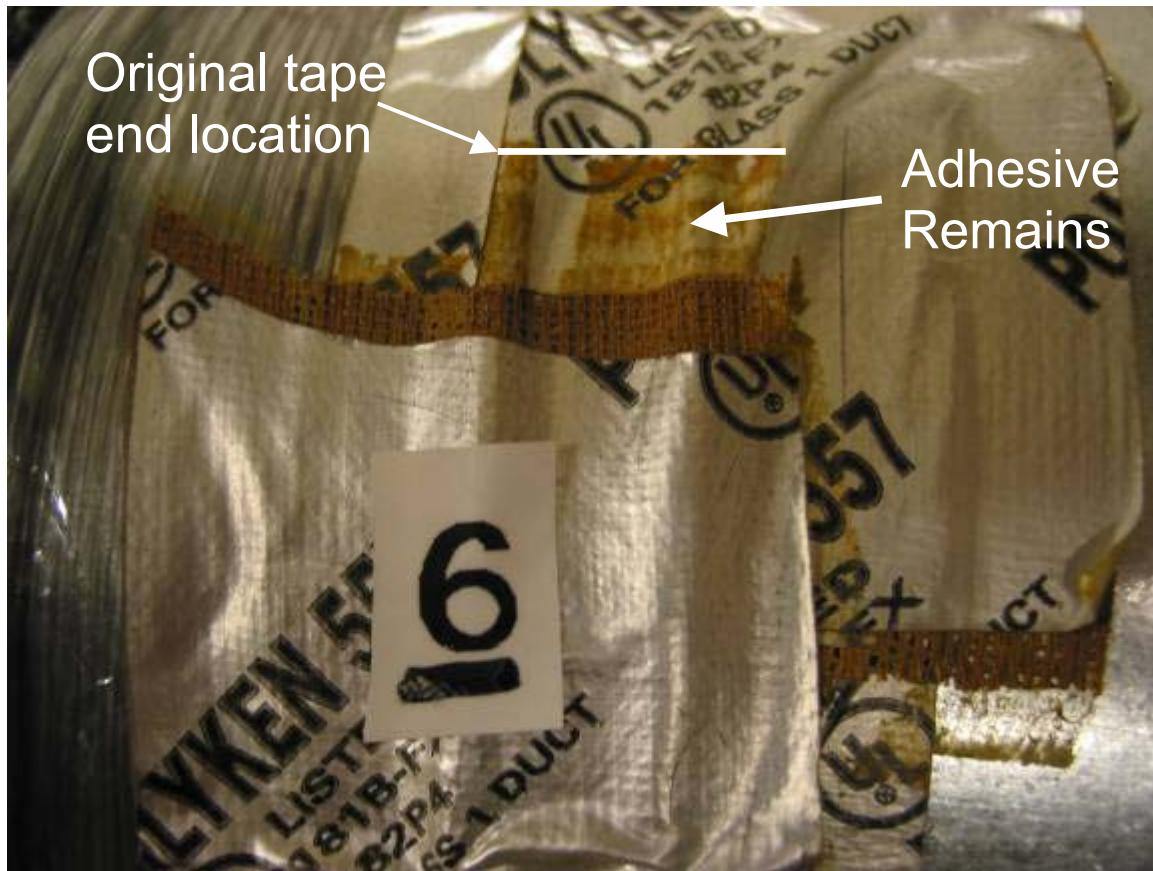
Figure A6. Sample 6. This figure is similar to Figure A5, but shows even more shrinkage.
