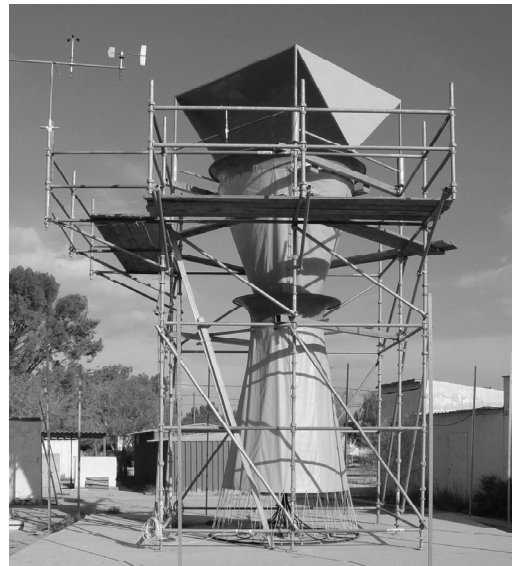
Figure 1: View of the prototype prior to installation of the wind baffle.
