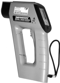
Figure 2: Infrared thermometer used for surface temperatures measurements.
