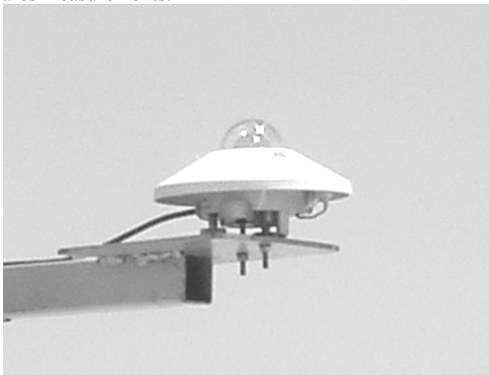
Figure 3: Piranometer utilized for measurements of solar radiation.
