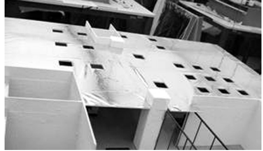
Figure 10: 3D physical model for daylighting, showing the plenum and openings to enhance daylighting and thermal performance.
