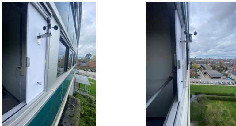
Figure 3: Measurement setup on the 1 st (left) and 10 th (right) floors of the high-rise building.
