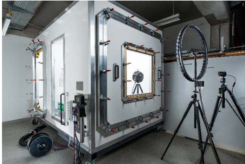
Figure 1: Test facility ATLAS equipped with its requisite measurement technology: Minneapolis DuctBlaster with Micro Leakage Meter (left), loudspeaker (inside), microphone array (right) and infrared camera (right)
