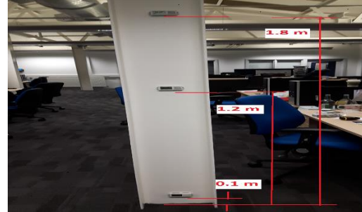
Figure 2: Schematic layout of the researchers' office at (CSEF) building and HOBO Temp/RH data logger location attached to the column at three different heights of 0.1, 1.2 and 1.8m
