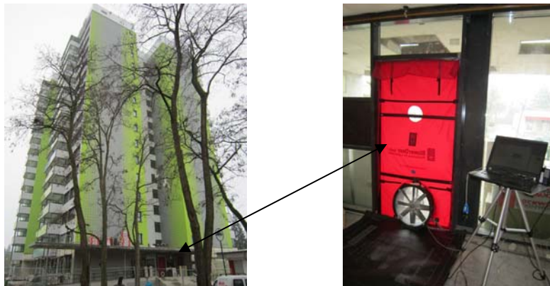
Fig. 1: Building view during the measurement in calm conditions (no wind). The measurements were conducted with a Minneapolis BlowerDoor Measuring System.
