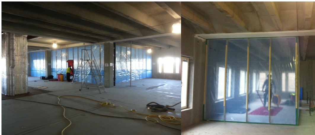
Figure 1. Different temporary boxes made with a stud frame and plastic film for early stage testing
