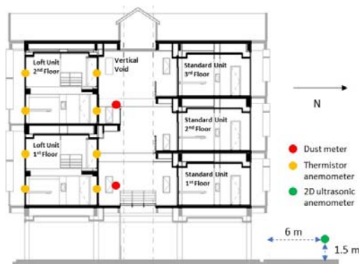
Fig. 4. Measuring positions of dust meters and anemometers.
