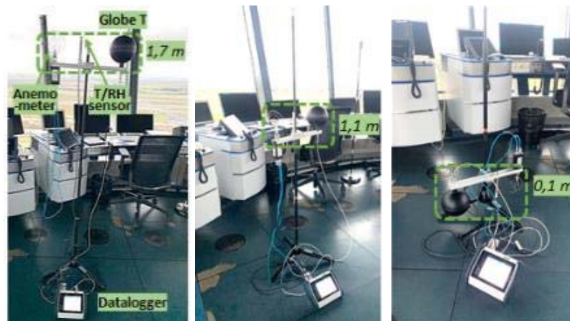
Figure 3. Thermal comfort monitoring station at the head, abdomen and ankle levels for a standing person including an omnidirectional anemometer, globe temperature, and air temperature and RH sensor
