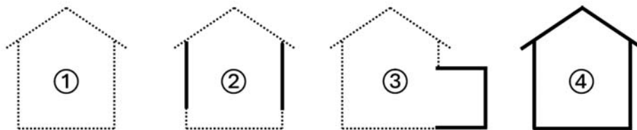
Figure 1: (1) Existing building (2) Partial renovation (3) Extension to existing building (4) Complete renovation (note on the graphic: lines with dots = not renovated; solid line = refurbished or new)
