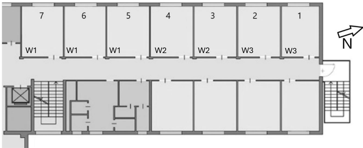
Figure 1: Lay-out of the ENEA living lab. The figure show the office number and the window typology in each room
