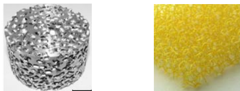
Fig. 2 Example of metal or plastic porous medium
