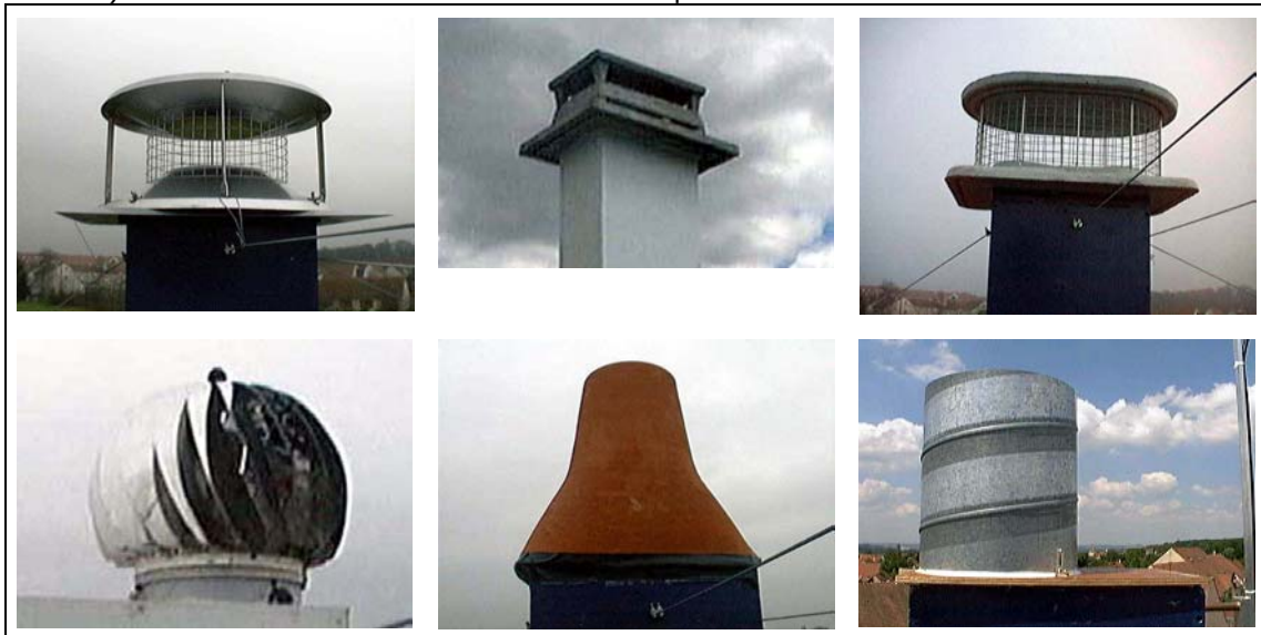
Figure 35 Cowls tested in the Photovent project
