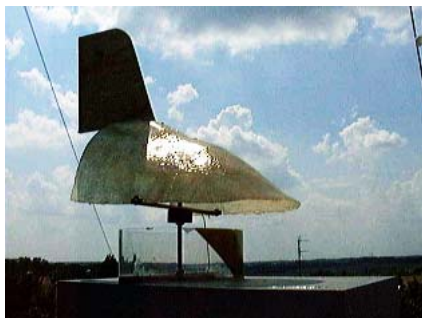
Figure 36 Rotating cowl developed in Photovent project
