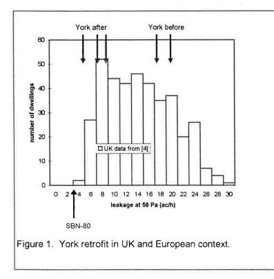
These results show a 2.5 - 3 fold improvement in air tightness in both sets of houses. This was brought about by a combination of measures, including draughtstripped replacement windows and doors, covering of tongued and grooved floors with 3 mm plywood sheeting (not sealed around skirting boards), and repair of obvious damage to plasterwork around doors and windows.
