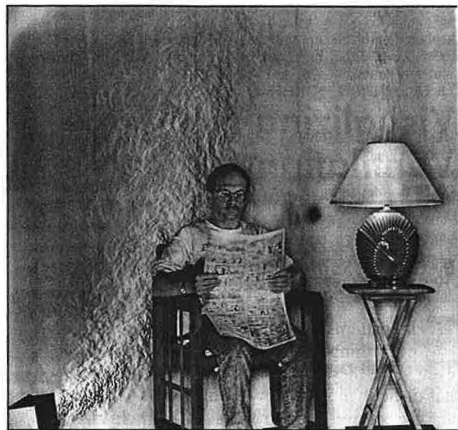
Figure 4: Full-scale schlieren photograph of a domestic room with person, lamp, and electric space heater.
