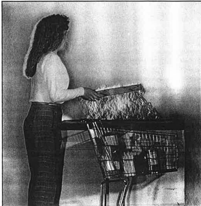
Figure 5: Full-scale schlieren photograph of a shopper removing a frozen pizza from a chest-type grocery store freezer.
