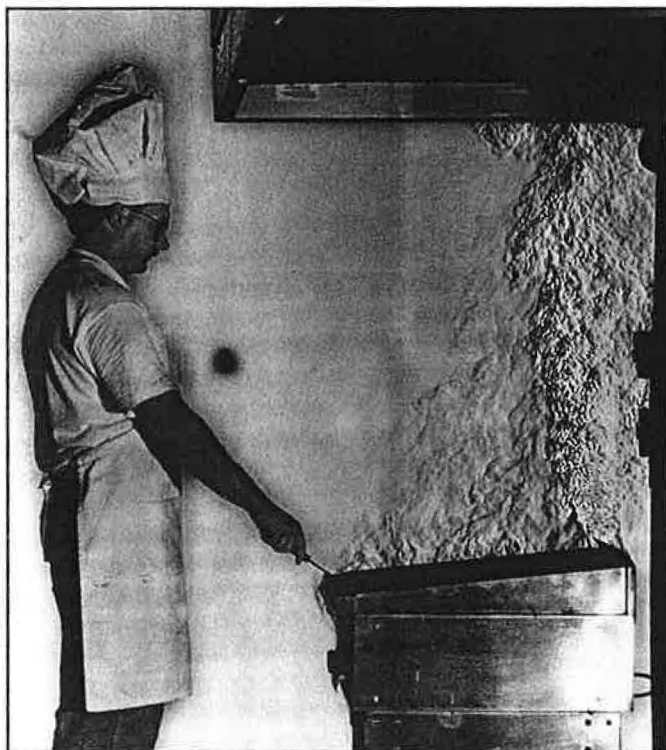
Figure 3: A commercial kitchen griddle and exhaust hood in use with cooking fumes made visible by the schlieren technique.
