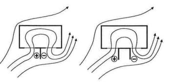
If the room has apertures on adjacent walls, wingwalls could considerably enhance crossventilation [9]. On the other hand, wingwalls modify the initial flow within the space.
