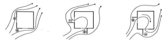
Vegetation can affect the air flow pattern in the same way as outside buildings or wingwalls [10]. Moreover, it also offer air filtering, noise reduction and shading.
