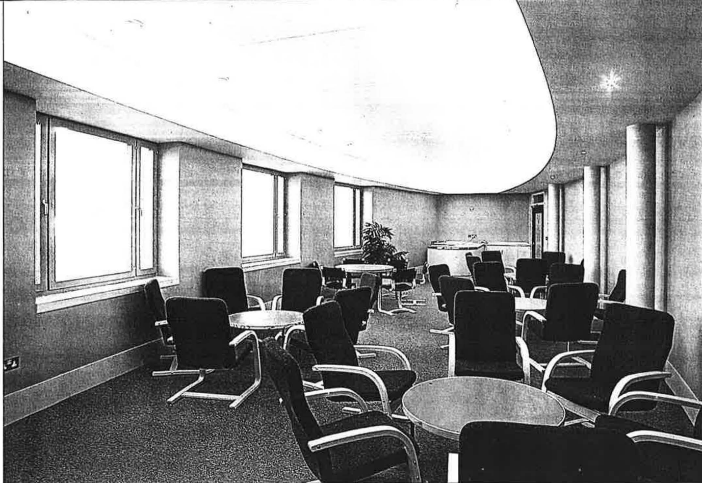
Even the general meeting and common rooms are well detailed. The windows are Swedhouse units with a mid-pane U-value of 1.3 W/m 2 K. This is the room above the main entrance, where the ceiling architrave mimics the curved north-facing wall. Nice room, pity about the wall colour.
