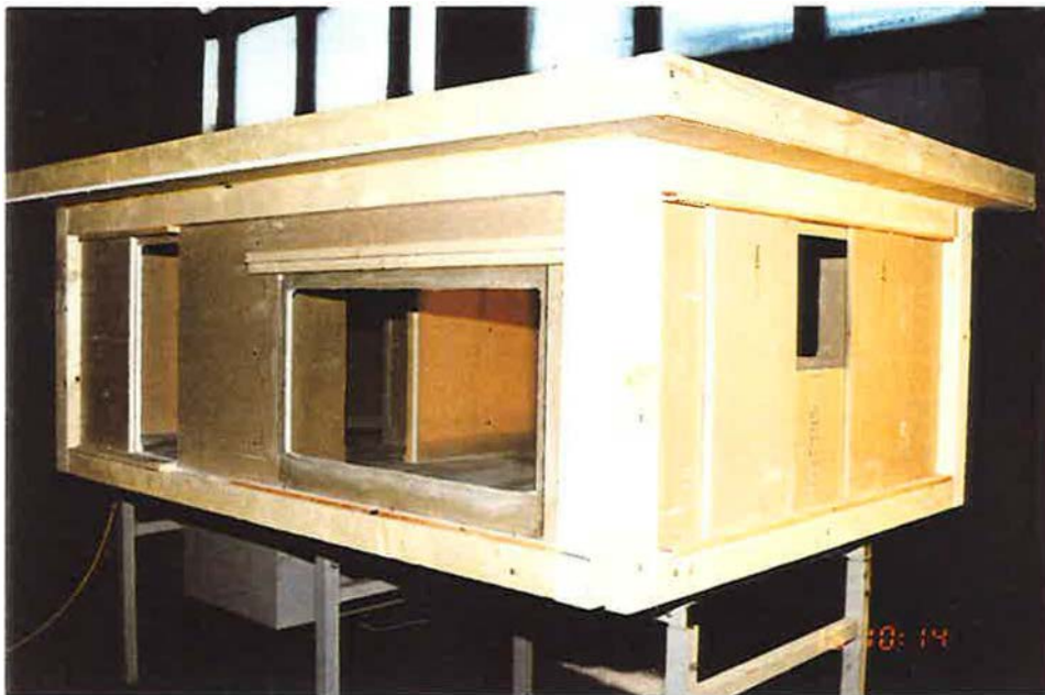
Figure 2. The first version of the test compartment from outside. In final tests the fire room walls were made of Siporex (see Figure 4), and there was no observation window in front because the tempered glass broke during the preliminary tests.
