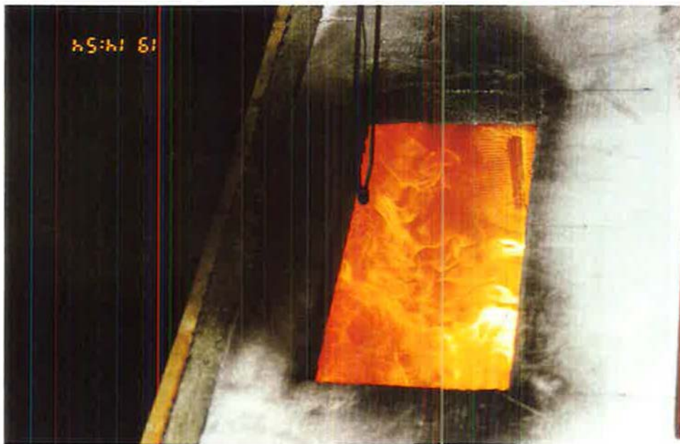
a) With natural through ventilation a flashover stage is reached in the fire room: the flames cover the whole room and momentarily also enter the entrance room. Hot gas layer forms in the fire room. (ST24)
