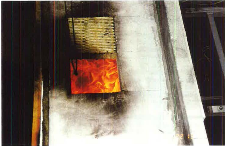
a) With the ventilation opening further away from the seat of the fire the flames extend outside as random, thin flames – if any. (ST36)
