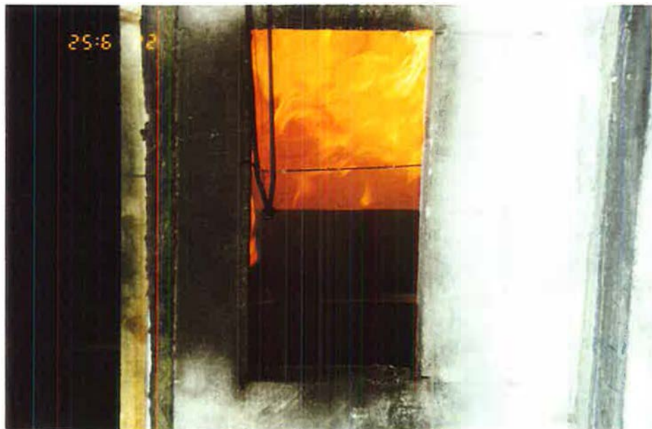
b) With PPV the gas layers and flames are mixed in the fire room. The flames are pushed away from the entrance door opening. (ST34)
