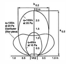
The flow pattern and throw are very important for the air experience in the room. The room temperature is 21 °C. The graph to the left shows some isovels for 0,2 m/s at 3 °C lower temperature and at different air flow.
