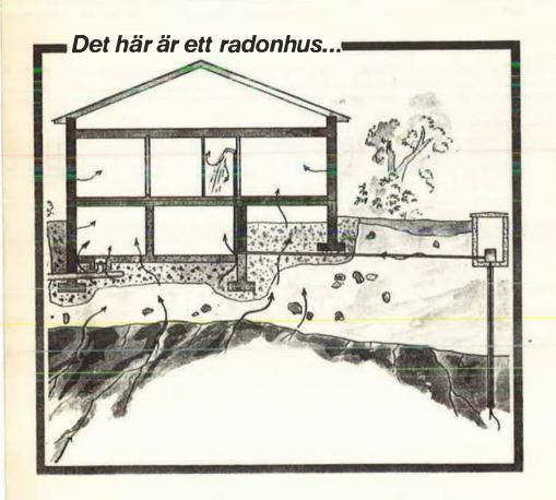
Figure 1. Illustration of the most common sources of indoor radon (soil, building materials and water) and its normal routes of entry. (Reproduced with permission from AIB Consulting Engineers, Solna, Sweden)
