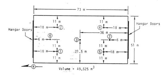
accomplished in 5 min. Accordingly, actual  $SF_6$  injection occurred for three passes around the hangar, or approximately 15 min. Initial calculations showed that an initial concentration on the order of 100 ppt could be expected.
