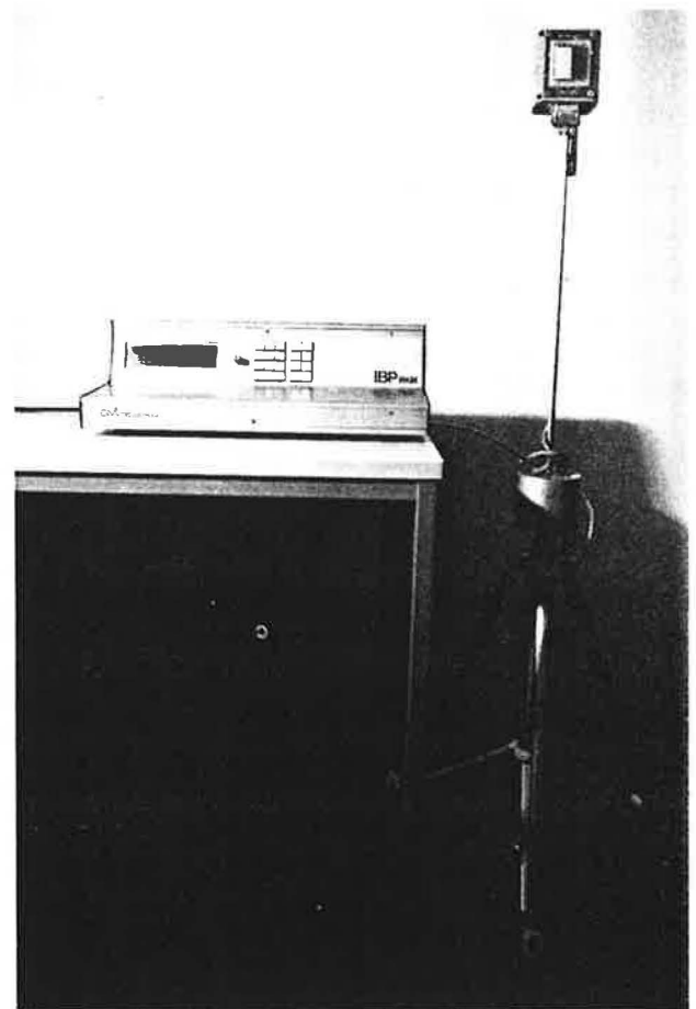
Fig. 3. Indoor climate analyzer consisting of the sensor mounted on a tripod with stepping motor, and electronics
