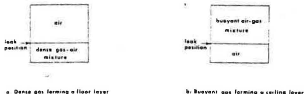
Figure 1. CONCENTRATION PROFILES IN AN UNVENTILATED ROOM UNIFORM LAYERS OF BUOYANT AND DENSE GASSES
