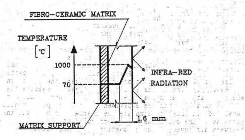
FIGURE 2 - Diagram of the temperature within the fibro-ceramic burner
