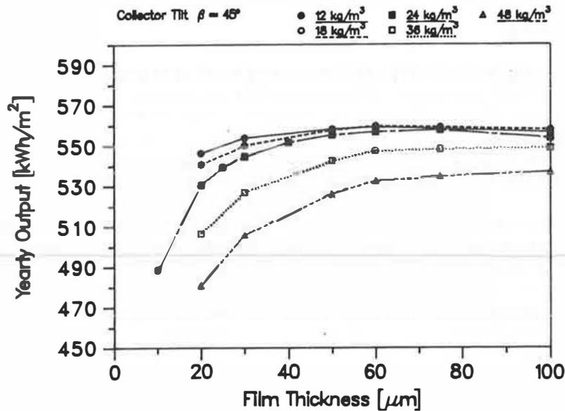
Figure 1 : Optimum mass distribution and film thickness
