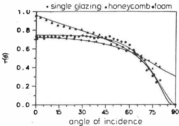
Fig. 1: Transmittance in dependence on the angle of incidence
