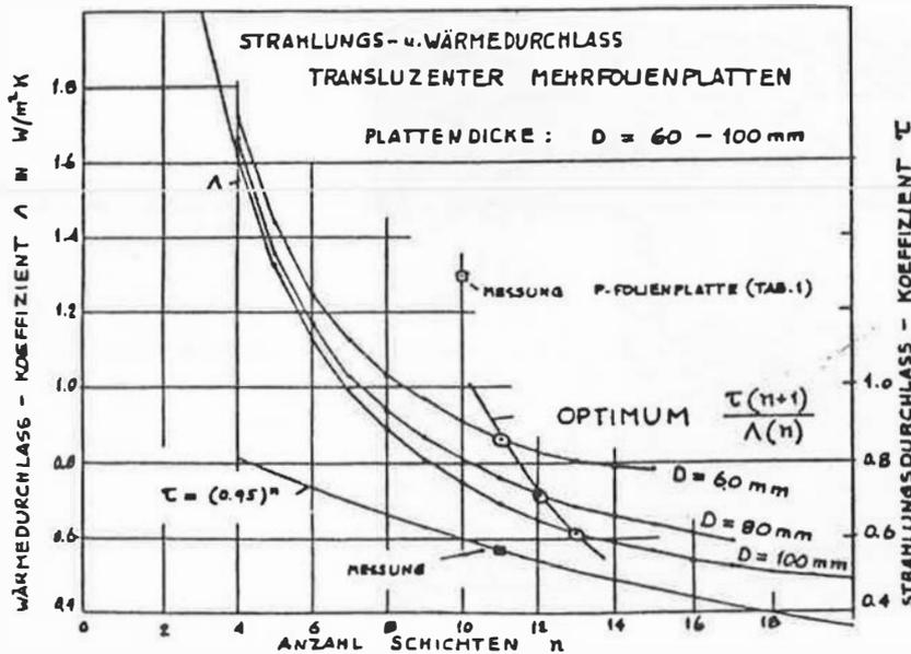
Fig. 5 Solar energy and heat transmission computed for P-layer insulation (cone angle  $60^\circ$ )
