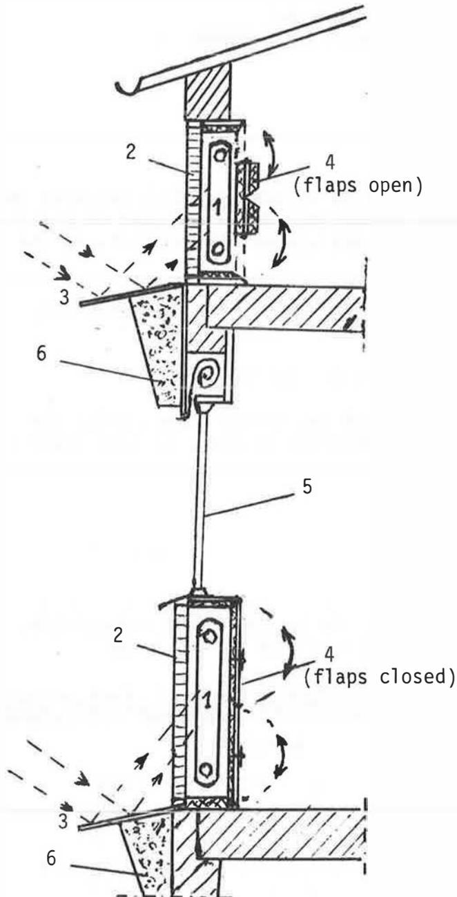
Figure: Integrated Solar Elements (ISE) in a facade
