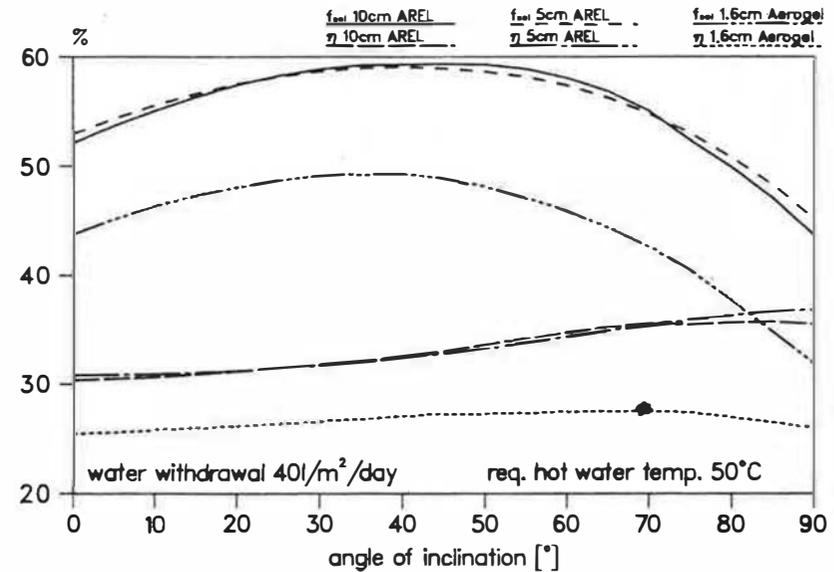
Fig. 6 Yearly solar fraction and yearly efficiency as a function of the angle of inclination, comparison of 3 different TIM covers
