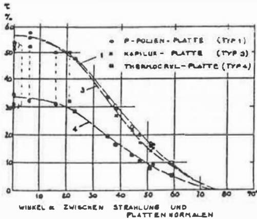
Fig. 4 Solar energy transmission of TI materials
