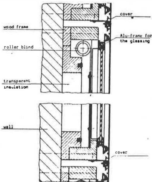
Figure 3: vertical section of the transparent facade module
