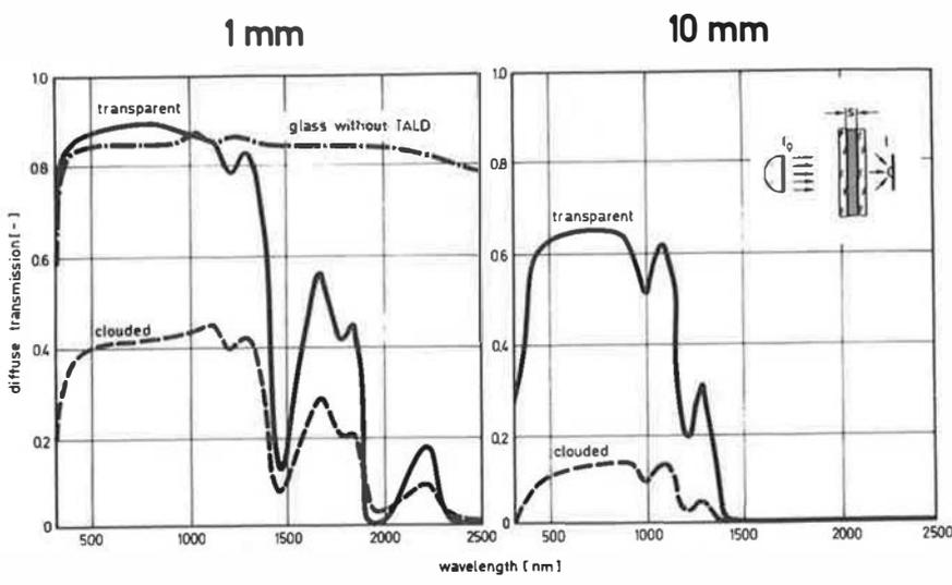
Fig. 3 Diffuse transmission of a TALD-Pane (clouding Temperature level 33°C) in transparent and clouded state for TALD gel layers of 1 mm (left) an 10 mm (right). In the visible range of solar radiation the transmission of glass without gel is lower than with TALD gel.
