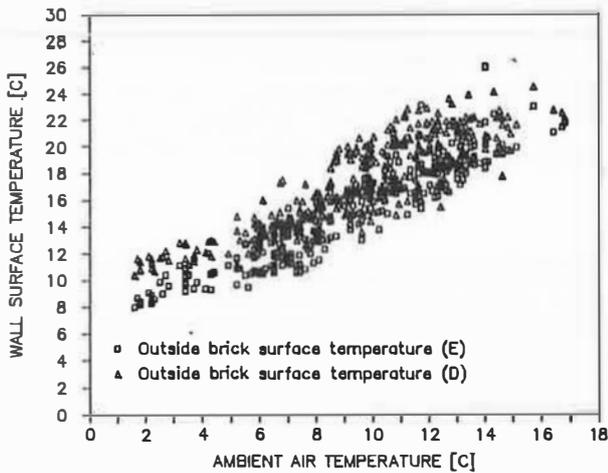
Fig. 5 West wall outside surface temperature: original data
