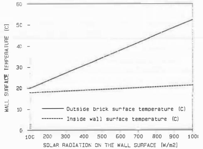
Fig. 4 South wall surface temperature: position C
