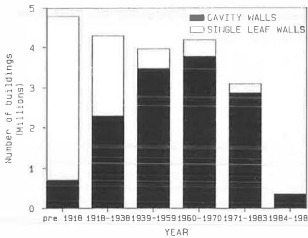
Fig. 1 Cavity walls in houses in the UK
