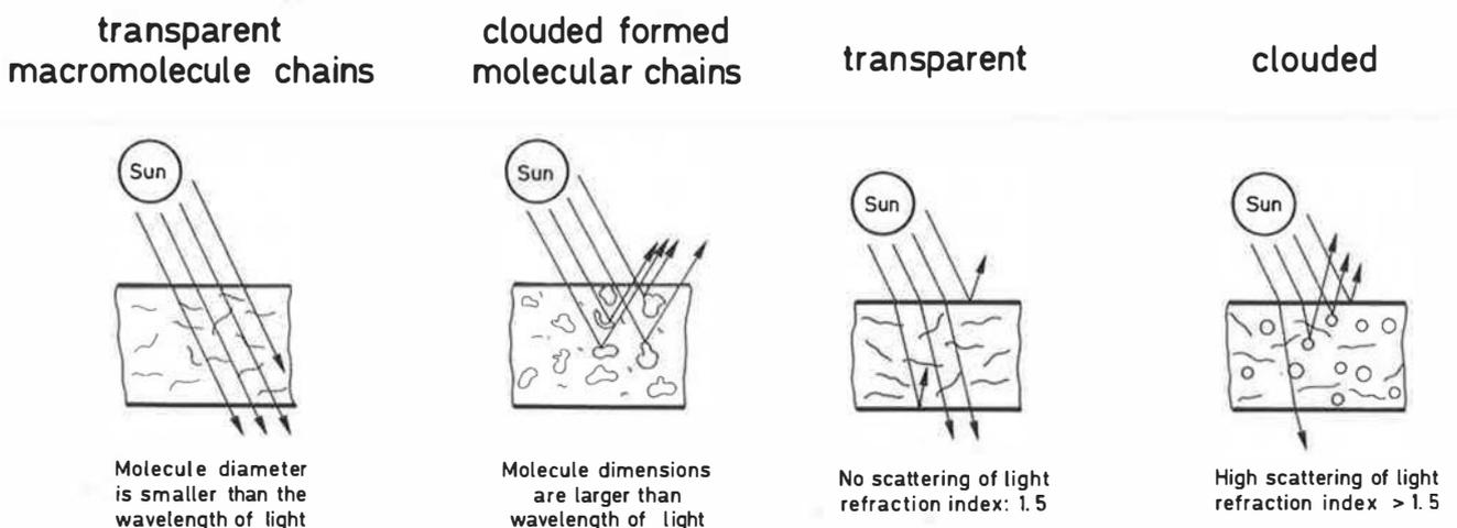
Fig. 1 Schematic presentation of the first clouding mechanism of TALD (left) depending on the molecular dimensions and the second clouding mechanism (right) occurring with the temperature dependance of water solution by means of polar interaction on wetting agents.
