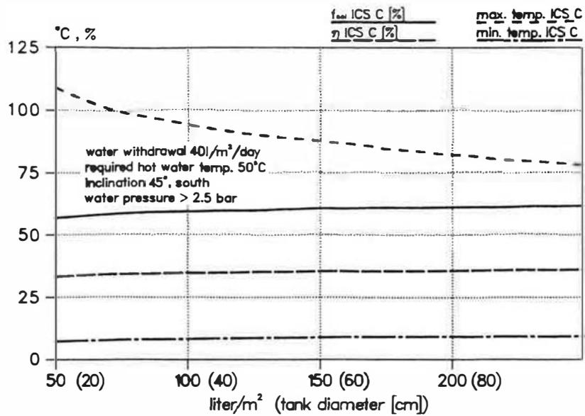
Fig. 3 Yearly maximum and minimum temperature (water withdrawal) of the ICS C, yearly efficiency and yearly solar fraction as a function of the amount of storage (water) volume per  $m^2$  absorber surface (tank diameter in parentheses)
