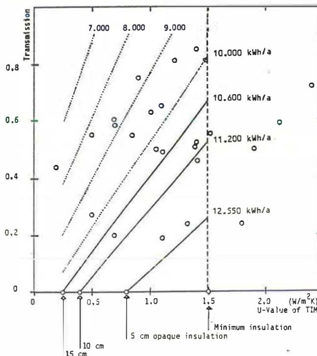
Fig. 1 "Curves" of equal auxiliary heating demand
