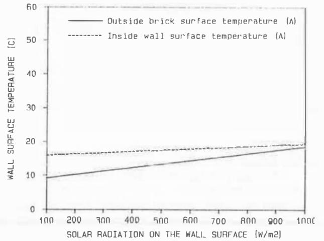
Fig. 2 South wall surface temperature: position A
