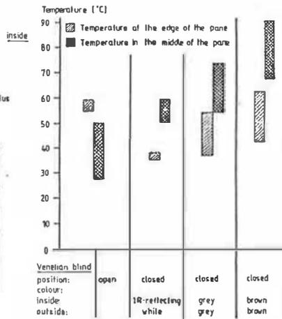
Fig.3 Temperatures of the pane next to the blind of the "Iplus"-glazing, dependent upon the position of the blind and the colour of the slats.
