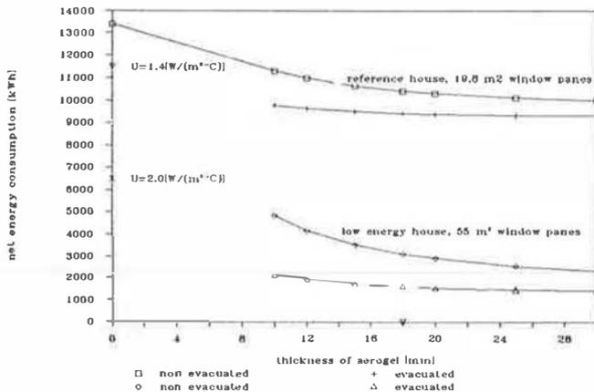
Fig. 3 Houses with aerogel window panes: computed annual net energy consumption
