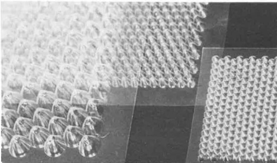
Fig. 2 P-layer samples with 5, 8 and 20 mm diameter cones and  $60^\circ$  cone angle
