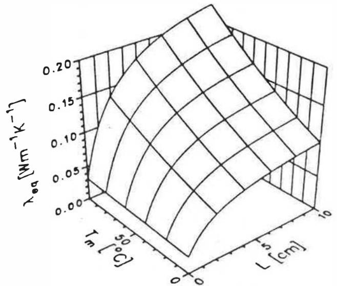
Fig. 2: Equivalent thermal conductivity of a honeycomb structure with  $\xi = 2$  cm as a function of the mean temperature  $T_m$  and thickness  $L$  of the material.
