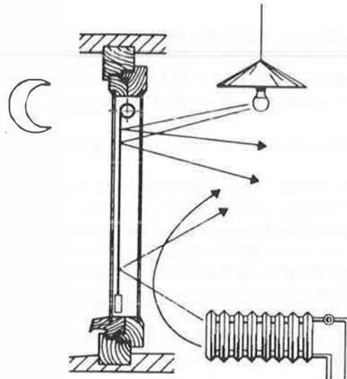
Figure 2: compound double glass window with integrated roller blind
