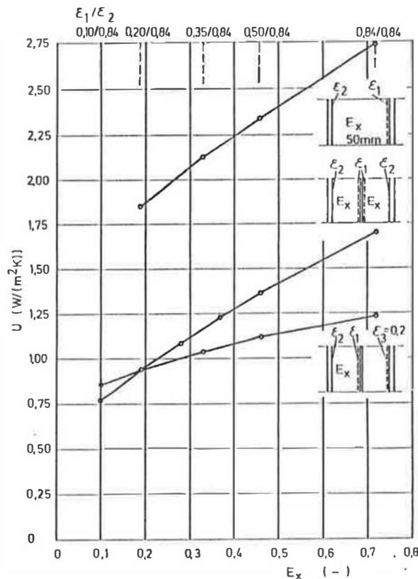
Fig. 3 Influence of the number of air gaps and their effective emissivity  $E_x$  upon the U-Value of window systems
