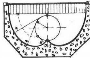
Fig. 2 Cross-section of optimised prototype (ICS C; tank: one single cylindrical unit with an involute reflector behind it)
