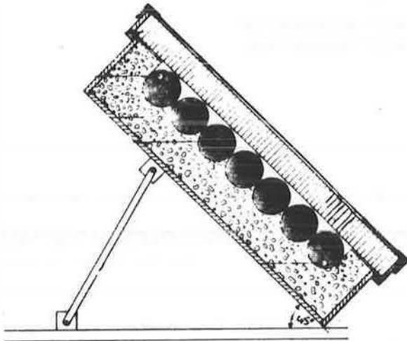
Fig. 1 Cross-section of the first prototype (ICS B; tank: 7 pressure-resistant subunits in series)
