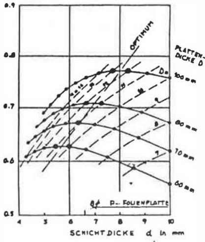
Fig. 6 Quality factor  $\tau/\Lambda$  as a function of layer thickness  $d$  and total insulation thickness  $D = nd$
