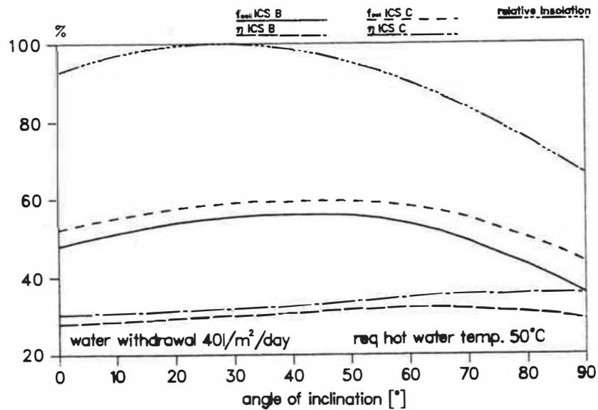
Fig. 5 Yearly solar fraction, yearly efficiency and relative insolation on the aperture as a function of the angle of inclination Comparison between ICS B and ICS C
