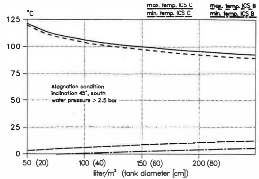
Fig. 4 Yearly maximum and minimum temperature of the ICS C and ICS B (stagnation condition), as a function of the amount of storage (water) volume per  $m^2$  absorber surface (tank diameter in parentheses)
