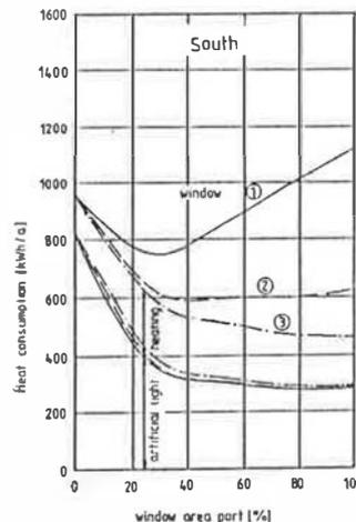
Fig.2a Heat consumption of the investigated windows, dependent upon the window area part.
