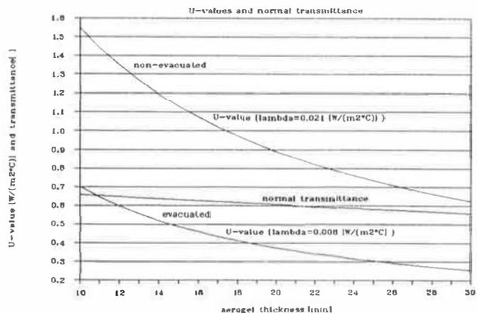
Fig. 1 Aerogel window panes: U-values and normal transmittance
