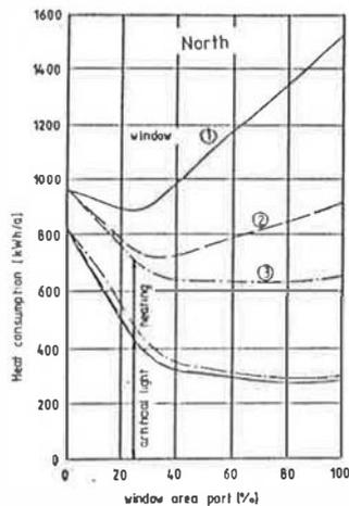
Fig.2b Heat consumption of the investigated windows, dependent upon the window area part.
