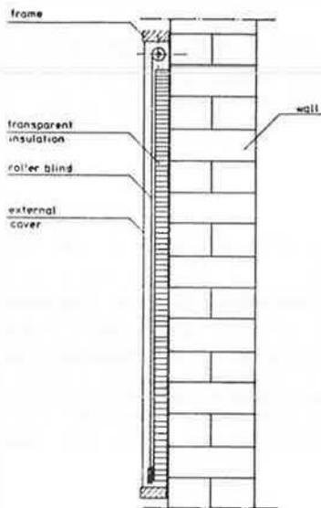
Figure 1: principle of the transparent wall insulation
