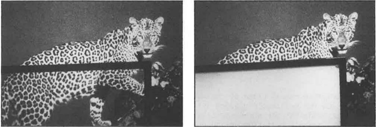
Fig. 2 Example of the transparent state of a TALD pane (left) and the same pane in the clouded state (right) at a higher temperature
