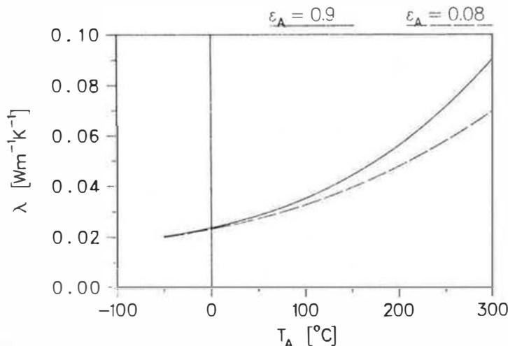
Fig.1.: Apparent thermal conductivity of a 2cm aerogel layer. The emittance of boundary A is  $\epsilon_A$  and of boundary B is  $\epsilon_B = 0.9$ .
