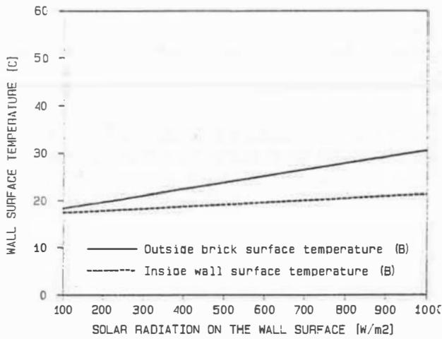
Fig. 3 South wall surface temperature: position B
