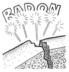
Common radon control methods include ventilation and source control to reduce entry of soil gases from the ground.
