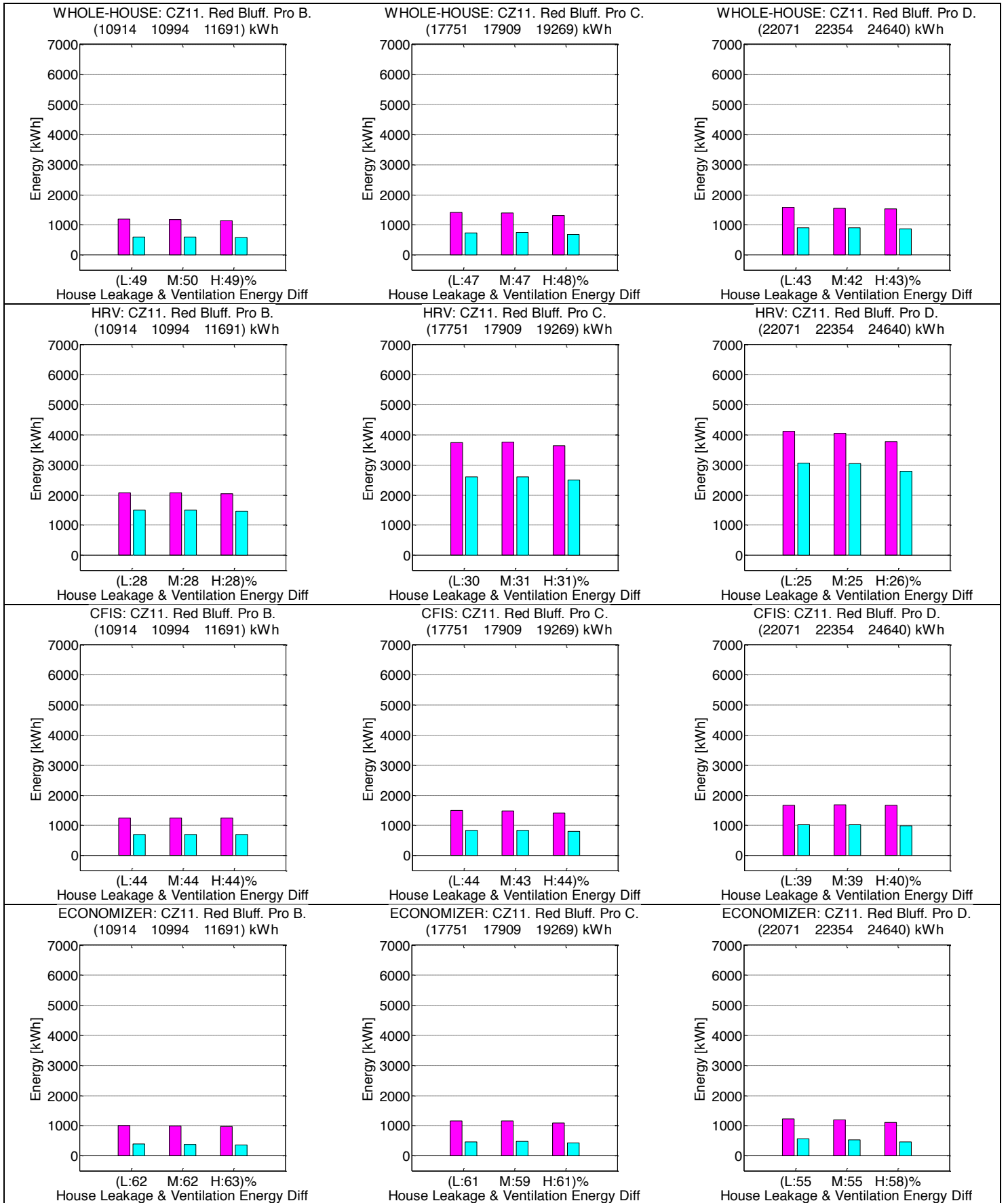
Figure 39: Ventilation-related energy penalty with and without RIVEC for climate zone 11, Red Bluff
