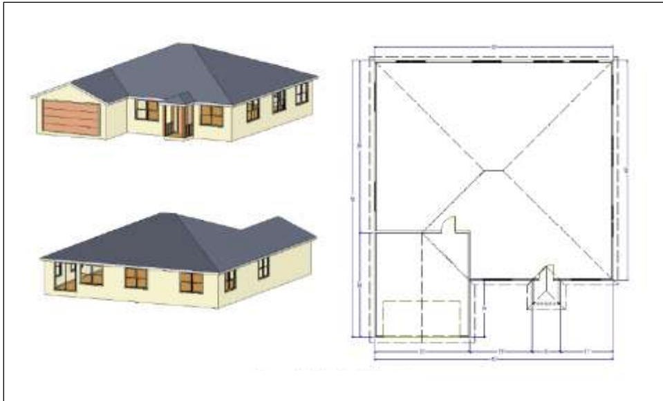
Figure 7: Title 24 Housing Prototype C (medium sized simulation house. The small house is a scaled down version of Prototype C) (Nittler and Wilcox, 2008)
