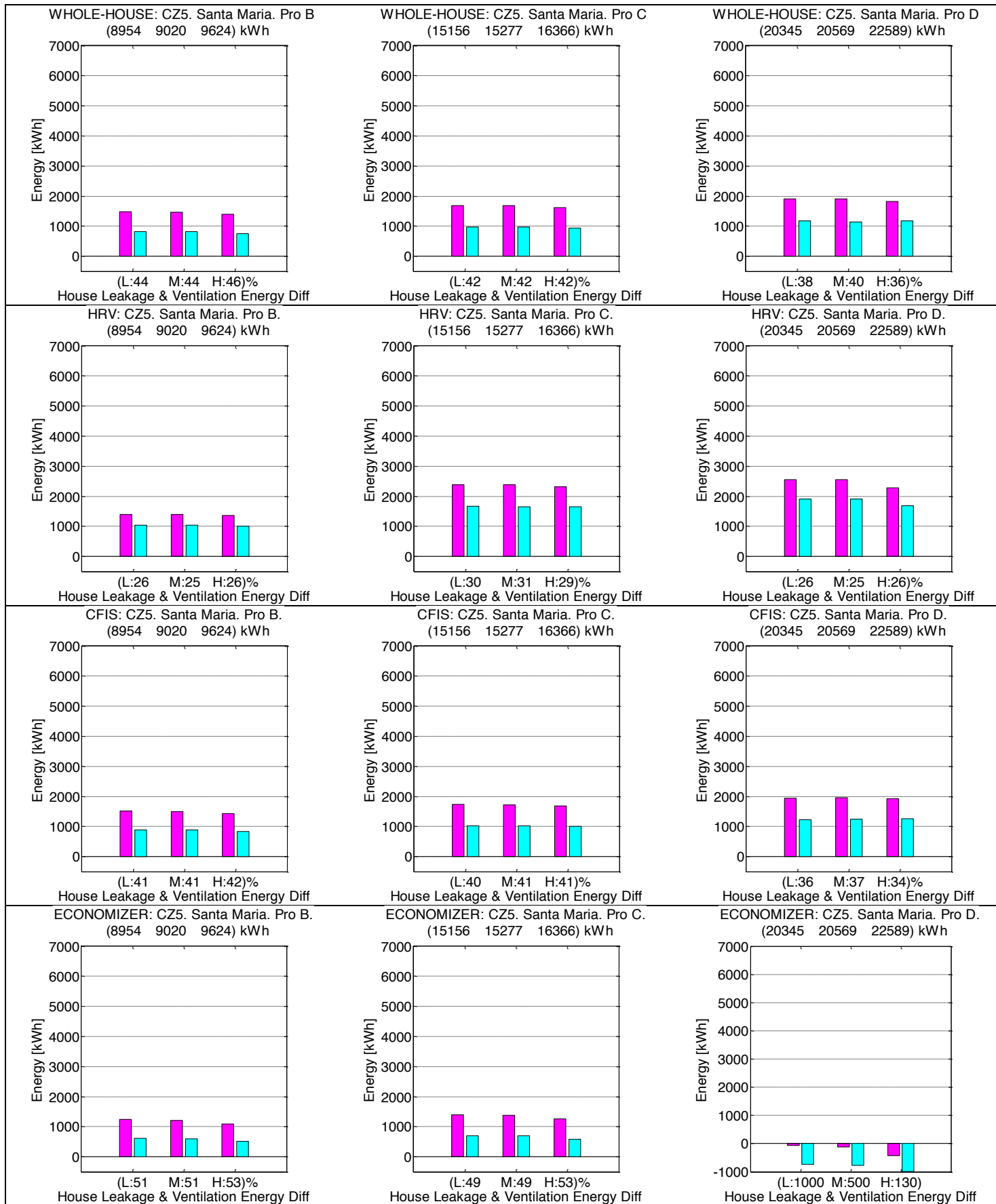
Figure 33: Ventilation-related energy penalty with and without RIVEC for climate zone 5, Santa Maria
