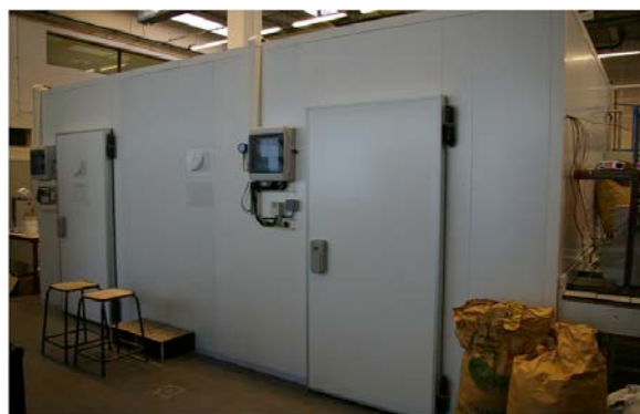
Figure 1 The biclimatic room at laboratory LIMATB of the "Université de Bretagne-Sud".
