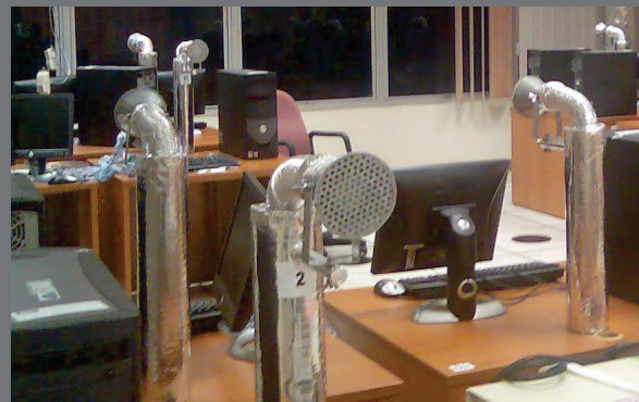
Field Environmental Chamber (FEC) experimental setup - Desk mounted PV with UFAD system
