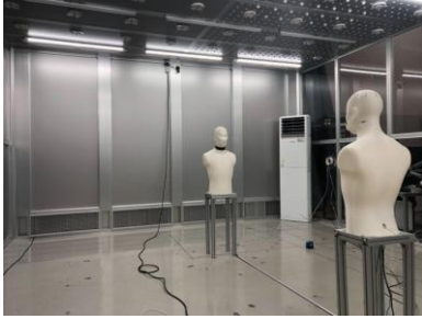
Figure 14: Experiment settings in the test chamber - Front-to-front (Shin H. W., Park, Park, & Kang, 2024)
